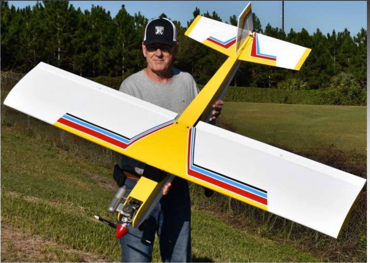
Don Riek with his scratch built Hobbystar 60 clone powered by a O.S. 65 LA
