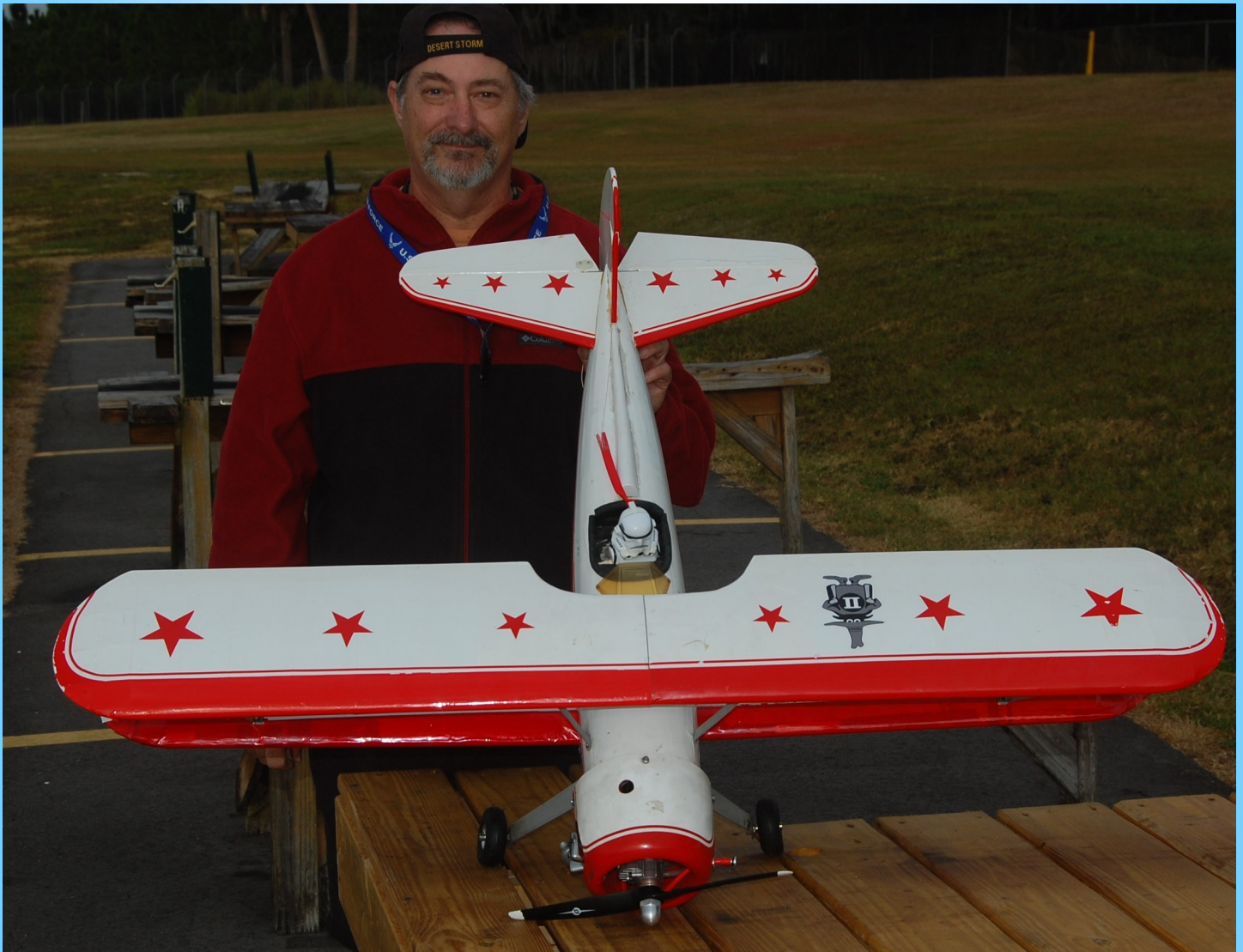
Devin Allen with his Kyosho Super Stearman powered by a Saito FA-62
